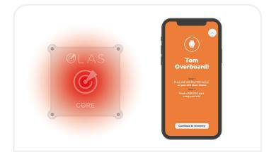
**4.** If testing with an OLAS Tag or OLAS Float-ON the alarm will occur after your set 'Alert Time' which has a default of 3 seconds. If testing with an OLAS T2 tag the alarm will occur immediately after it is switched off.
