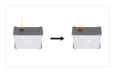
**9.** Press the control switch once. The Core will beep, the number of beeps represent the number of tags it is now tracking. Tracking resumes. Solid red on the control switch indicates it is tracking correctly.
