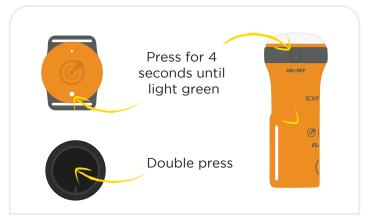
7. Switch the OLAS transmitter back ON.
