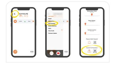
**4.** If using an OLAS T2 go to 'Alert Settings' in the menu and select the alert function for the OLAS T2. Now when you switch off your OLAS T2 tag it will activate the alarm immediately.
